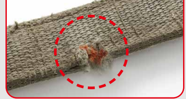
Damage in the width direction
